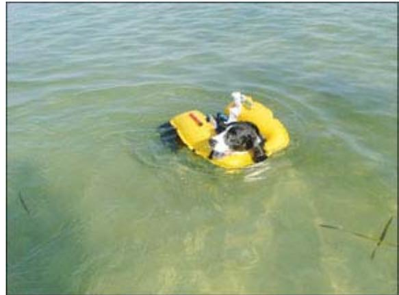
**The Critter's Inflatable pet PFD, with its 25 pounds of buoyancy, kept the chin of the PS test pooch high out of the water. The vest's inflating device can be set to operate automatically or manually.**
